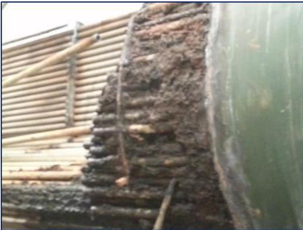
**Figure 3: Old Heat Exchanger Corrosion**
