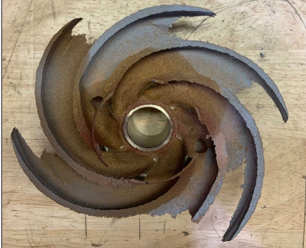
Primary pump's degraded impeller
