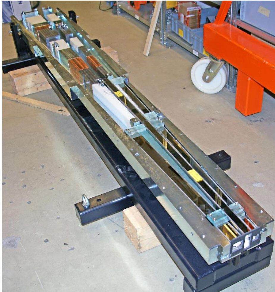
In-pile cold neutron guide assembly – Fabrication Phase
