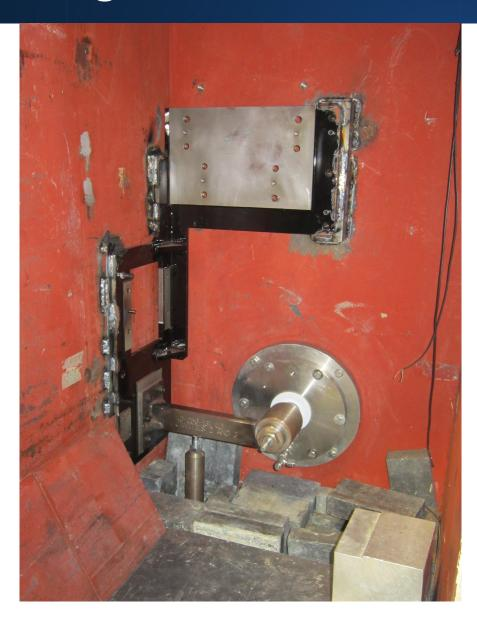
Steel frame with pins designed and fabricated in house
