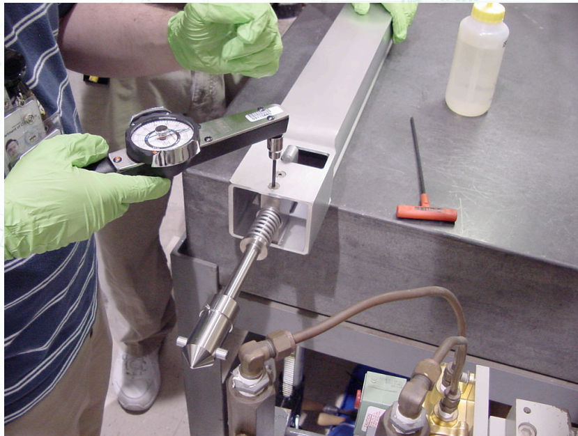
▶ ATTACHING TRANSFER HEAD TO FUEL ELEMENT
