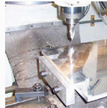
g) Since U/Mo foil is contoured, top of pressed plate must be machined to be flat
