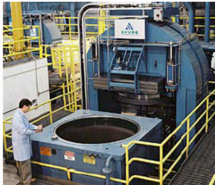
f) Hot isostatic pressing of U/Mo, Zr, Al clad and borated Al if inner plate
