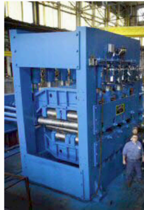
b) Contoured rolling of U/Mo foil
