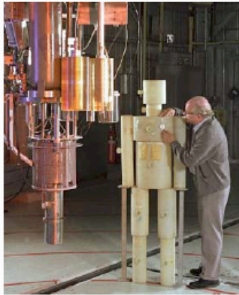
a) Health Physics Research Reactor fuelled with U-10Mo alloy
