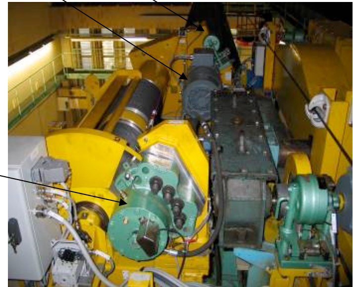
Safety brake on rope drums
